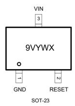
The package of IMP809xEUR/T is SOT23, with pin assignment shown in following table:
