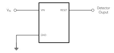
Detector output remains low if V<sub>IN</sub> is below detecting level, and jumps to high if VIN is above detecting level for 240ms
