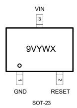
The package of CS809x is SOT23, with pin assignment shown in following table:
