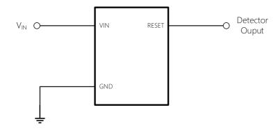
Detector output remains low if  $V_{IN}$  is below detecting level, and jumps to high if VIN is above detecting level for 240ms
