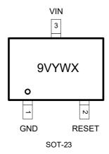
The package of CN809x is SOT23, with pin assignment shown in following table:
