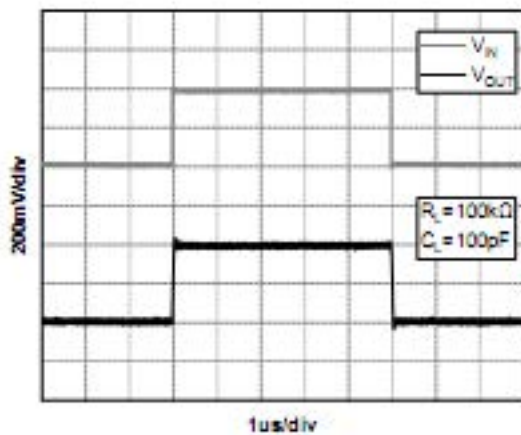
Figure 6. Small-Signal Step Response( V_S=5 )
