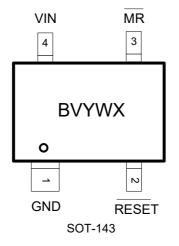
The package of SGM811 is SOT-143, with pin assignment shown in following table:
