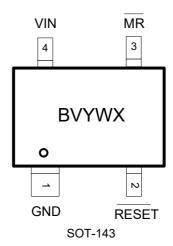
The package of CS811x is SOT-143, with pin assignment shown in following table:
