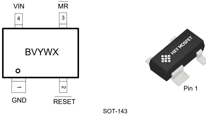
The package of CS811x is SOT-143, with pin assignment shown in following table:
