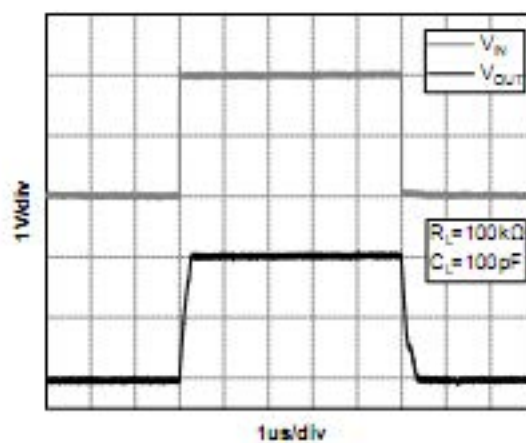
Figure 7. Large-Signal Step Response( V_S=5\text{V} )
