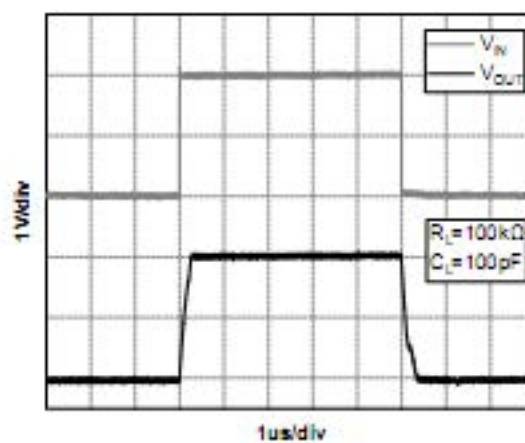
Figure 7. Large-Signal Step Response( V_S=5\text{V} )
