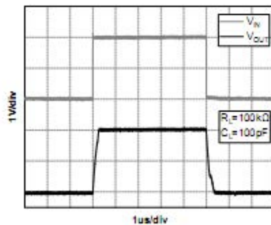
Figure 7. Large-Signal Step Response( V_S=5\text{V} )
