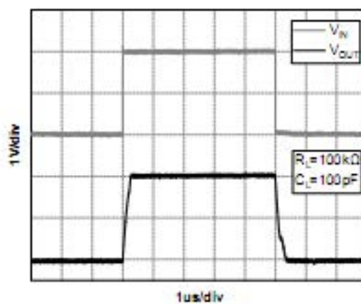
Figure 7. Large-Signal Step Response( V_S=5\text{V} )
