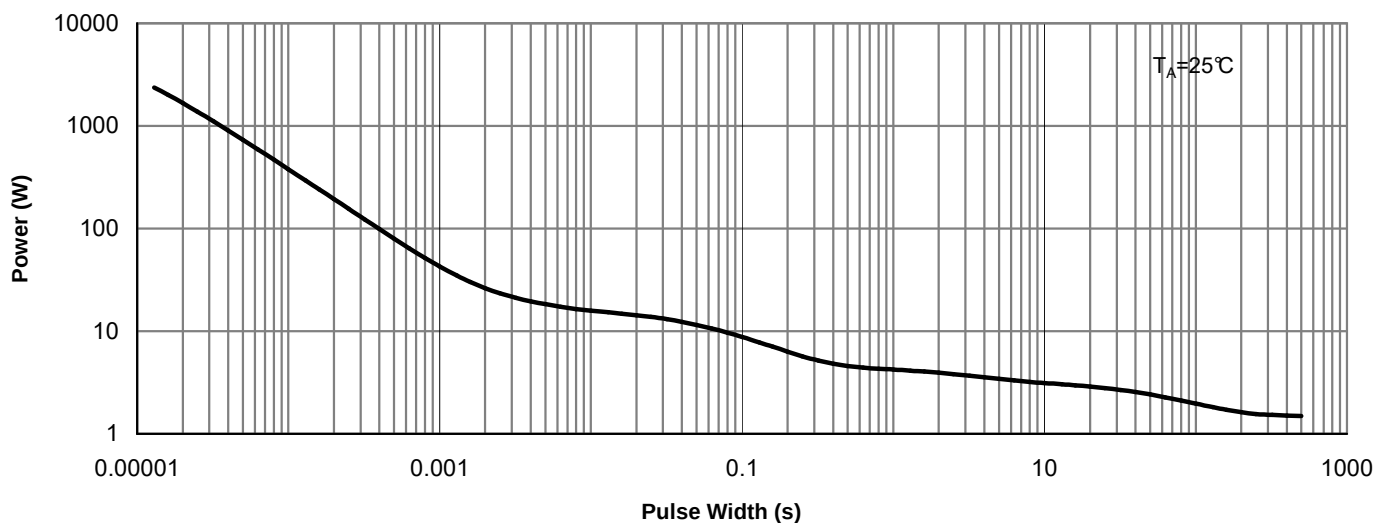
Figure 11: Single Pulse Power Rating Junction-to-Ambient (Note F)
